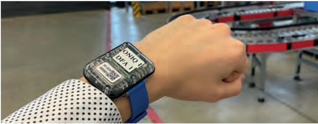
Figure 3: Transponder from Ubisense on the wrist
