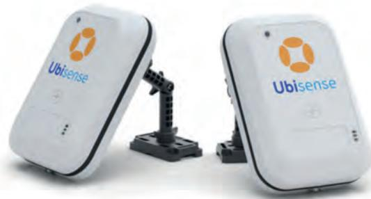
Figure 2: Antennas for the RTLS from UbiSense
